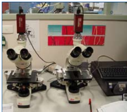
SiroMat automatically scans across the slide.
