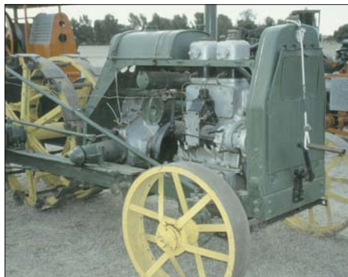
The two cylinder diesel engine can be clearly seen in this view of the off side of the Benz Sendling. (Photo IMJ)
