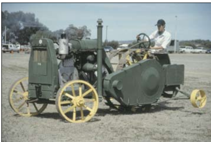
This Benz Sendling is one of the finest remaining examples of these rare tractors. It is one of the many fascinating exhibits at the Booleroo Steam and Tractor Preservation Society in South Australia. Note the guard covering the final drive chain and the outrigger stability wheels. (Photo IMJ)
