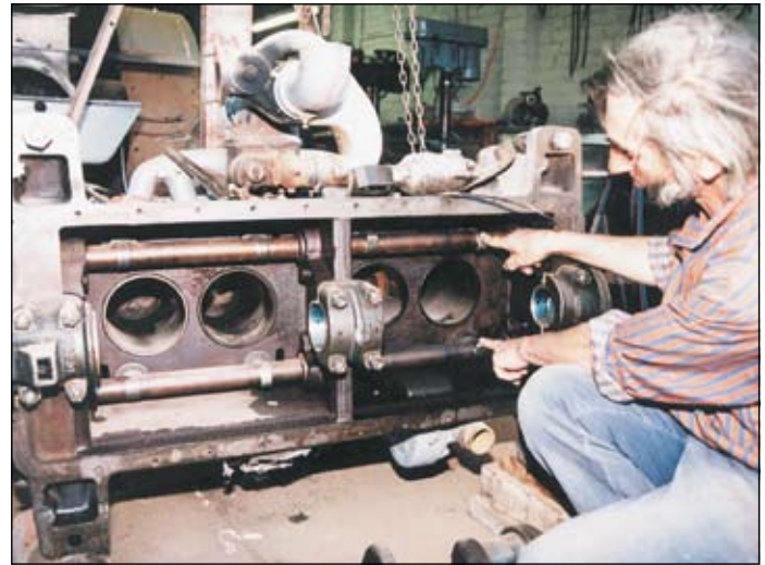
Pictured is Newton Williams pointing out the twin camshafts of the 16 valve four cylinder engine as fitted to the Twin City 27-44. (Photo IMJ)
