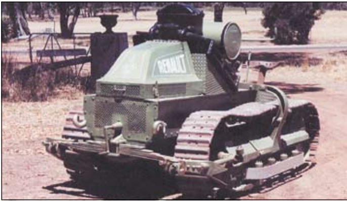
The Renault GP/HI crawler was the most expensive tractor at Trangie. Derived from a World War One tank, this French crawler was a very capable unit with a drawbar pull well in excess of what might be expected with regard to its size. Notice from the text that at Trangie it pulled two ploughs in tandem. This example is part of the Victorian Redhill Museum collection.
