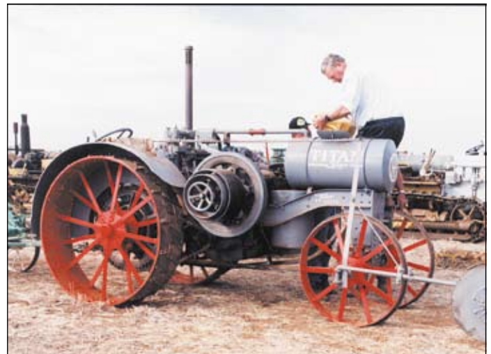
This International Titan 10-20 was photographed at "Plough and Be Counted 2". Although costing half as much again as the Fordson, its performance at Trangie, in 1922 could not match that of the cheaper machine. During the test the two cylinder Titan went through 310 gallons of cooling water in 61 hours and 56 minutes!
