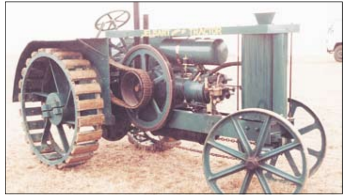
The Jelbart was the sole Australian tractor to be put through its paces at Trangie and the only single cylinder tractor to compete. It was described as being of eight horse power, which was possibly correct, being dependant on the governed rpm. Remarkably it ploughed the most acres per hour. The Jelbart pictured was seen at the 1997 Ausplough, and is part of the Cunnington collection.
