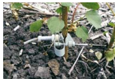
FIGURE 1: Stem micro-variation sensor in situ and the logger with antenna for remote download
