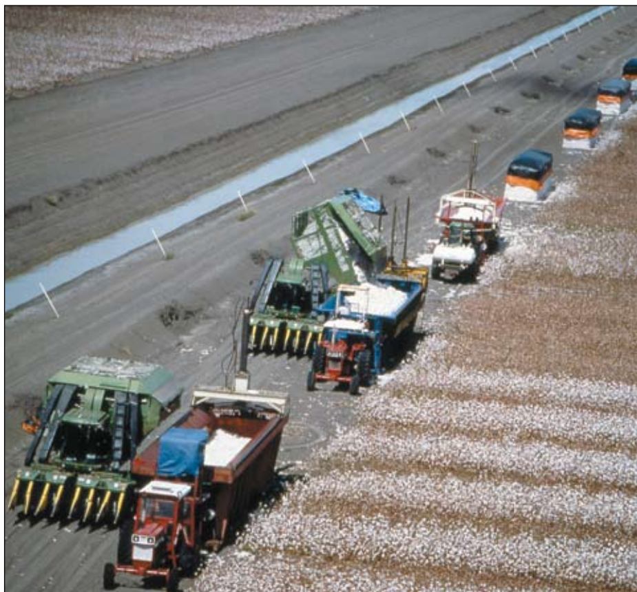
Pickers and module builders can be dangerous around power lines.
