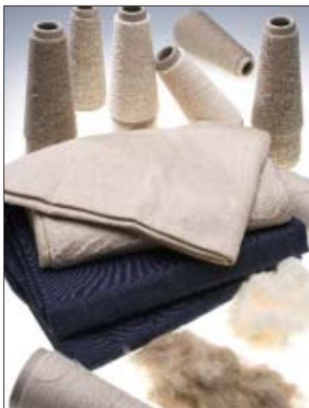
Samples of raw flax (darker fluff) and raw cotton (lighter fluff) and yarns, woven denim, and knitted fabrics made with various blends of cotton and flax.
