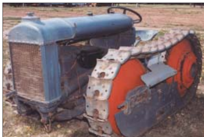
Several North American manufacturers designed after market crawler track gear, for fitting to the Fordson Model F. Pictured is a Model F, owned by Norm Bates of WA, equipped with tracks manufactured by the Bell City Mfg Co, Racine, Wisconsin.
