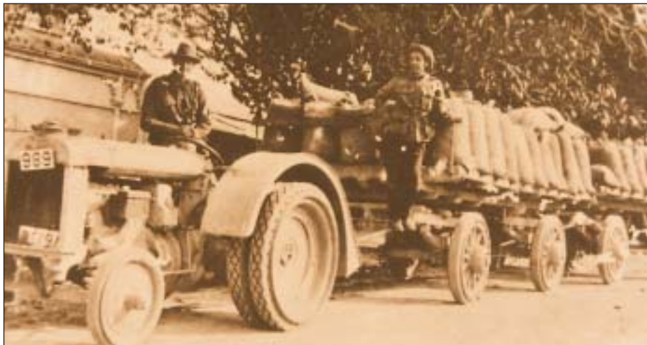
A historic photograph of an industrial version of the Fordson Model F, complete with solid tyres, hauling two converted horse carts loaded with salt. The photo was taken at Edithville, SA.
