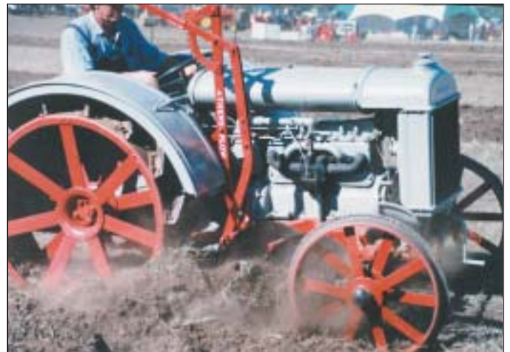
A Fordson Model F, fitted with an Athens mid mounted twin disc plough, taking part in a vintage tractor ploughing competition in Victoria. The owner and driver is Mal Brinkmann.
