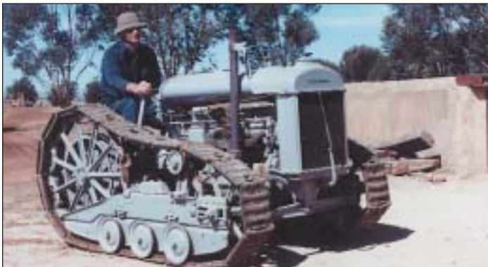
This 1924 Fordson Model F is mounted on a pair of Trackson crawler tracks, a product of The Full-Crawler Co, of Milwaukee, Wisconsin. The diameters of the rear driving sprockets are the same as the steel wheels they replaced, thus providing the equivalent driving speeds. The tractor pictured is part of the world-class collection of tractors at the Booleroo Steam and Tractor Preservation Society Inc. of South Australia.
