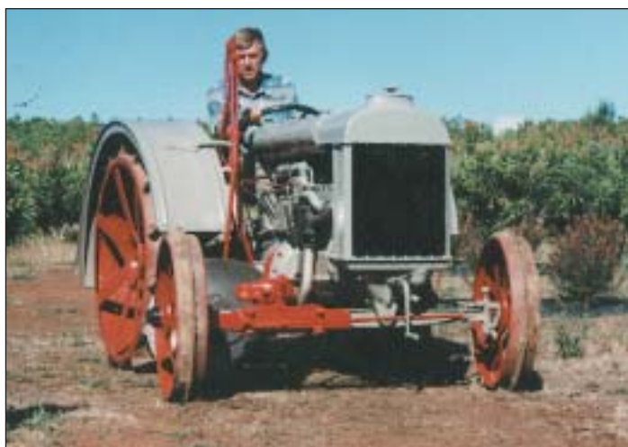
Another view of Mal Brinkmann's Model F illustrating the extension to the front axle, required to make space for the two furrow disc plough.
