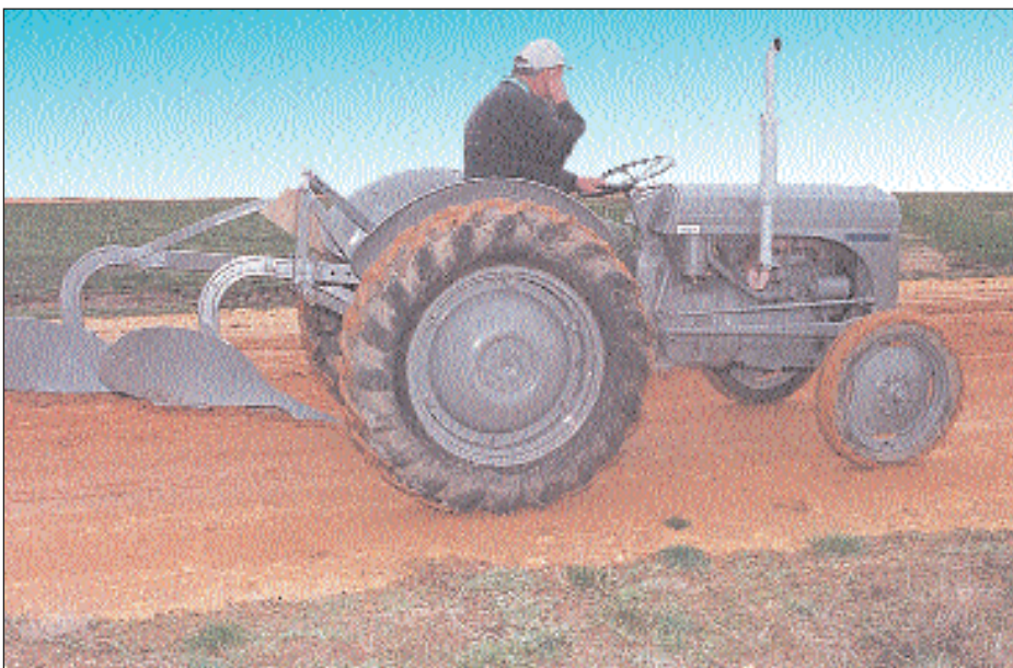
Harry Ferguson claimed: "A tractor on its own is worthless. A plough on its own is worthless. Put the two together and you have a system of farming." Prior to the introduction of Ferguson's patented weight transfer principle, a two furrow 12 inch mouldboard plough (as pictured) would have required a tractor of twice the weight of a Ferguson to obtain the traction necessary for its operation. (Photo I.M.J. taken at Lake Goldsmith, Victoria)
