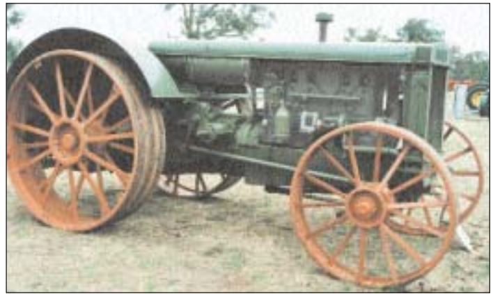
Pictured is a 1928 Huber 22/38 Super 4, No. 9048, belonging to Australian collector Les Burns. The tractor is provided with two forward speed and one reverse gear. Note that for transportation purposes the steel grips have been removed from the wheels. (Photo IMJ)
