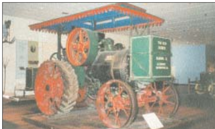
Pictured is a 1910 30 hp Huber Steam Traction Engine, with a boiler shell diameter of 44 inches and a thickness of 0.375 inches. Thirty steam flues of 101 inches had a diameter of 2.5 inches. The unit weighed around 12 tonnes. Huber steamers were highly regarded and compared more than favourably with their other North American counterparts. (Photo courtesy W. Johnson)
