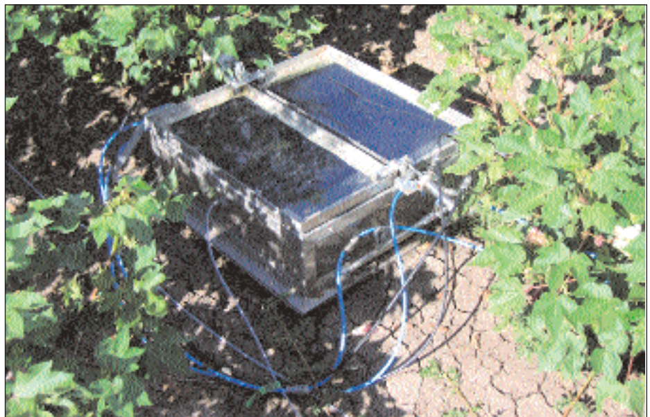
Measuring greenhouse gas emissions with gas chromatographs
