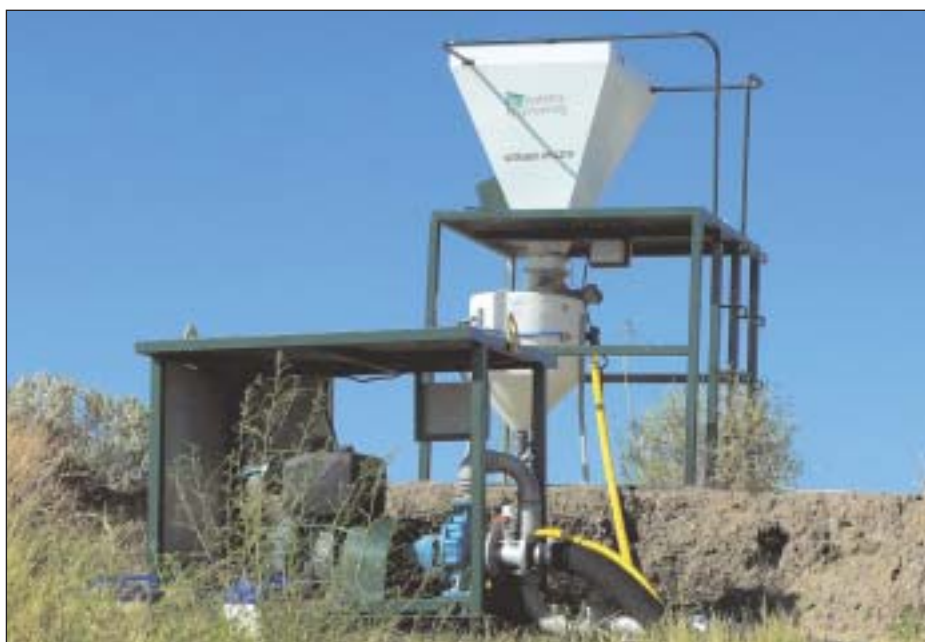
Mixing hopper used to mix the chemical monolayer.
