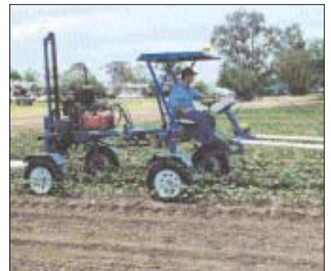
An EM31 mounted on a ATV and connected to a GPS system.
