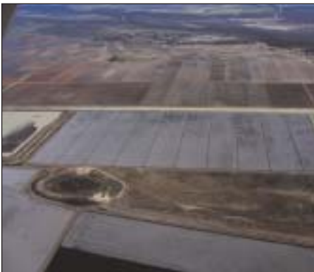
Conventional irrigation at the bottom of picture, bankless channel (centre) and new BC development at the top of picture.
