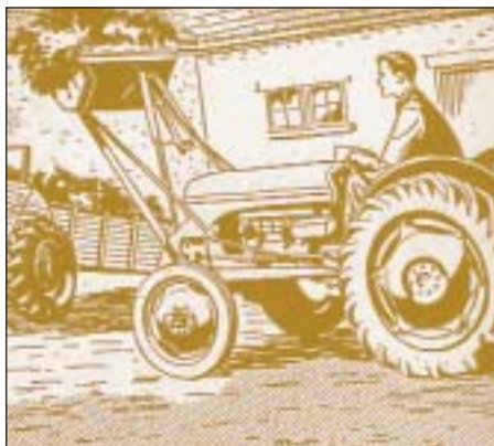
The Ferguson Manure Loader was operated by a series of links connected to the three point linkage system. It was capable of raising 1000 lbs of dung, sufficiently high to load into the spreader.
