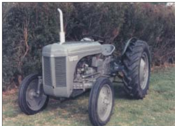
The Ferguson TE Series was introduced in 1947 and for over a decade was Scotland's number one selling tractor. It incorporated the Harry Ferguson patented three point linkage, which revolutionised mechanised agriculture. This restored example is owned by A. Latimore. (Photo I.M.J.)
