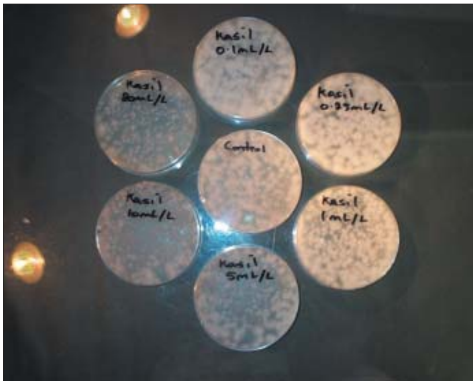
Reduced growth rate of Fov after five days when a conidial suspension was mixed with potassium silicate at five, 10 and 20 ml/L and spread onto solid growth media. There was no effect at 0.1, 0.25 and 1.0 ml/L compared to the untreated control.
