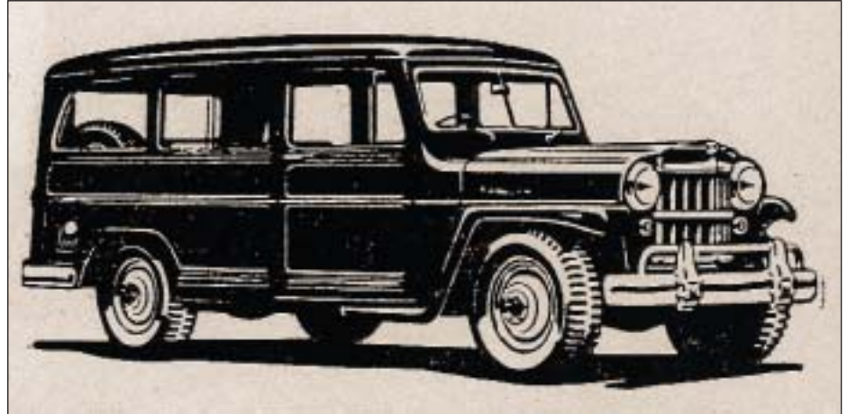
Mr McMullet's pride and joy was a 1963 Willys Super Hurricane Jeep station wagon, powered by a six cylinder engine of 115 bhp. The American Willys Jeep range was assembled at Rocklea, Queensland, by Willys Motors Australia Pty Ltd, and distributed in NSW by York Motors and in Western Australia by British Tractors and Machinery Pty Ltd.
