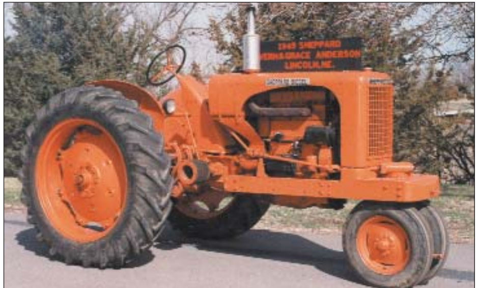
The SD 3 was the top seller of the Sheppard Diesel range. Its three cylinder diesel produced 32 belt hp. This row crop example is part of the Anderson Collection, located in Lincoln, Nebraska. (Photo IMJ)
