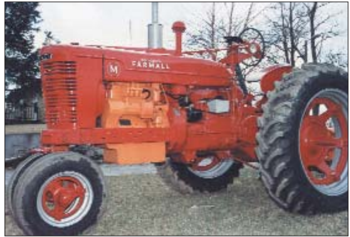
Pictured is an International Farmall M repowered by the purpose built replacement three cylinder Sheppard diesel. (Photo IMJ)
