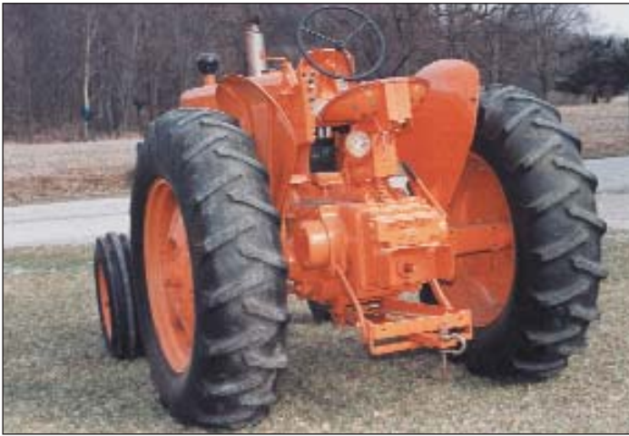
This rear view of the SD 4 illustrates the outboard disc brakes and the commanding operator position. (Photo IMJ)
