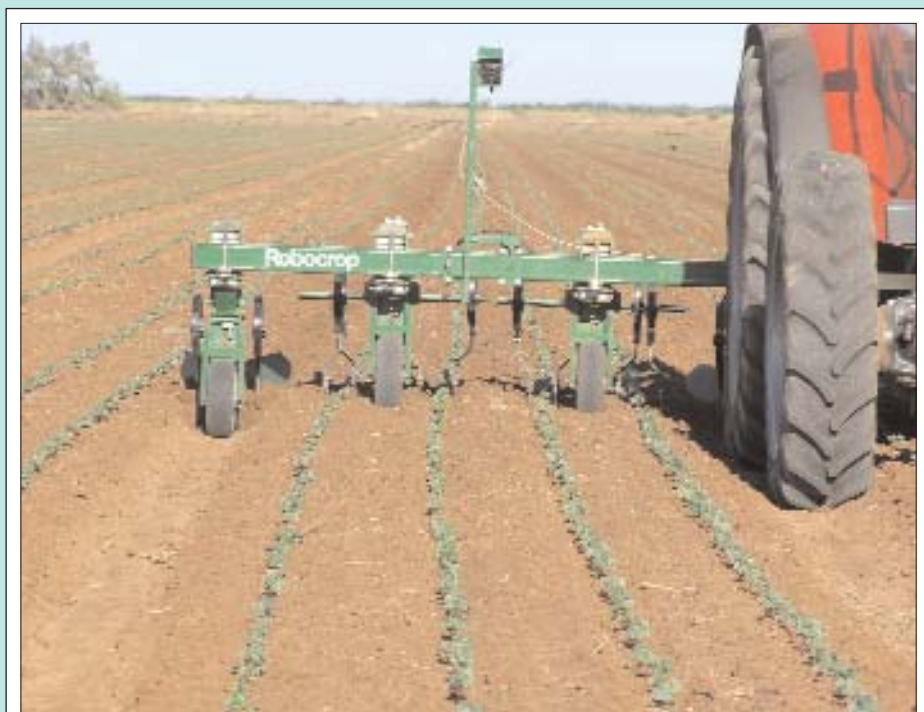
The robotic weeder cultivating at 10 km per hour in narrow row (15 inch) cotton in southern NSW.
