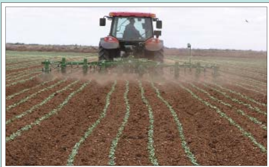
A real-time video image of the crop ahead allows the machine to follow curves, correct for GPS errors, or follow contours in dryland crops or headlands.
