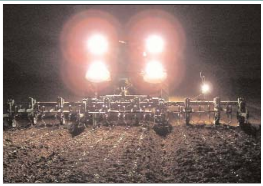
Robotic weeding works well at night, enabling 24 hour operation at critical times.
