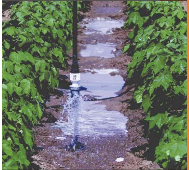
Senninger Irrigation's LDN when used with the Bubbler Pad converts to a LEPA device from a spray applicator.
