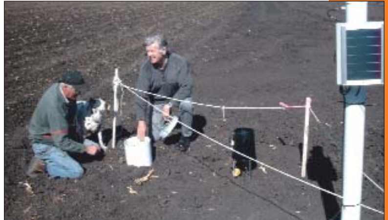
The deep drainage recording equipment with Stewart Leadbetter, at left, on his "Cabarita" cotton farm near Pittsworth and NRM's Des McGarry.
