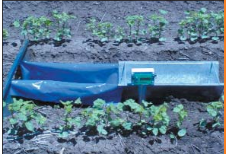
The depth of flood irrigation can be measured down the length of the field.
