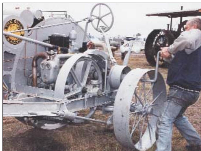
Considerable effort is required by Norm Johnston to crank the Big Bull's 20 hp engine with its two horizontally opposed cylinders. Note that the right hand rear wheel, through which the crank handle is inserted, is purely an idler balancing wheel. (Photo I.M.J.)
