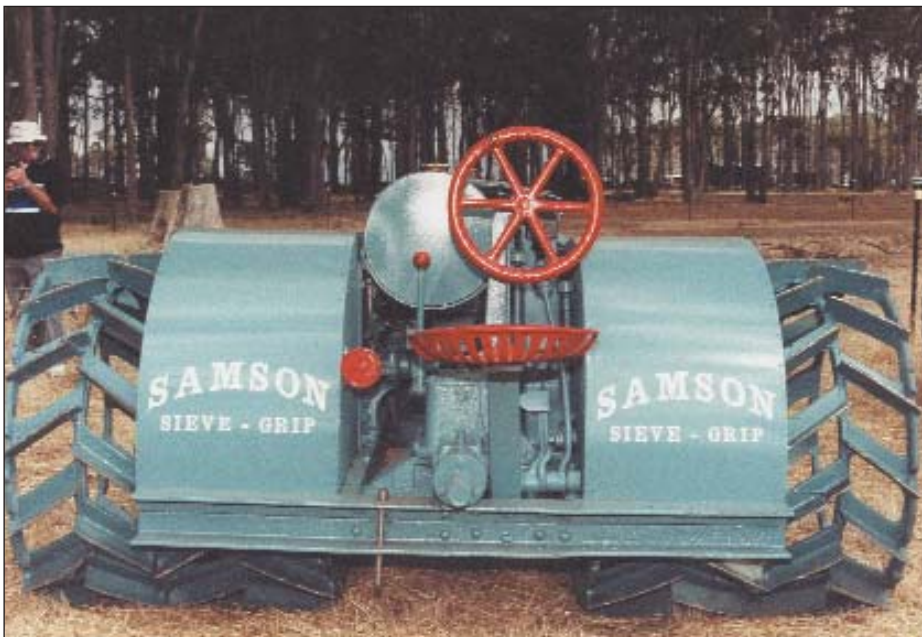
This rear view of the Samson Sieve Grip illustrates the patented design of the driving wheels. Although appearing perhaps elementary in their construction, the Samson wheels with their open slats were unique, as they did not clog with mud or clay, a common problem with conventional steel tractor wheels. (Photo I.M.J.)
