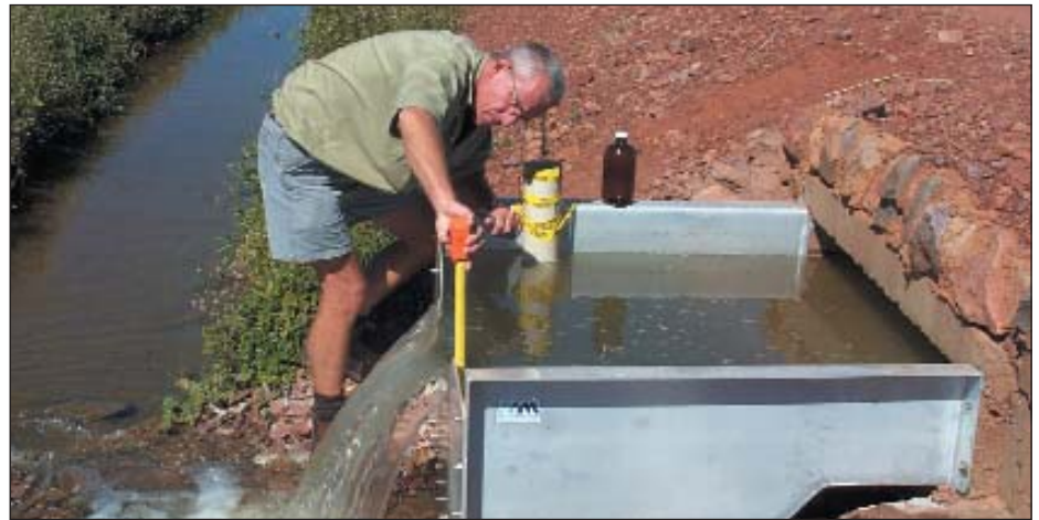
John Moulden measuring water quality off the field and the volume of tail water.
