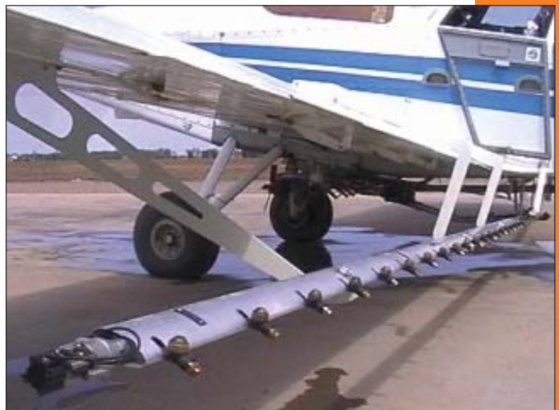
The JARBA Boom showing the capacity of the nozzles to be rotated in flight for droplet size control. (Photo courtesy Jones Air)
