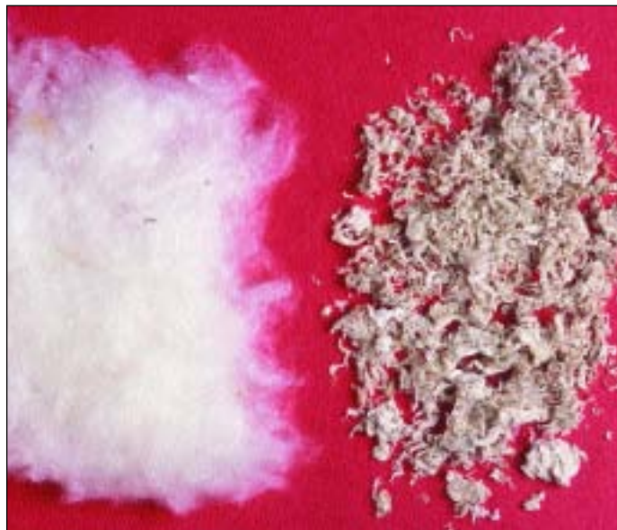
Untreated cotton fibres (left), and regenerated nanocomposite fibre containing seven per cent clay.
