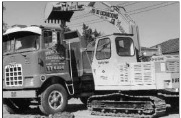
The Furukawa FH2A was also imported into Australia and indeed was the first lightweight hydraulic excavator seen in this country. The unit pictured was purchased by Reg Lee Excavations and proved to be the most reliable item of earthmoving equipment in his extensive fleet. (Photo I.M.J.)
