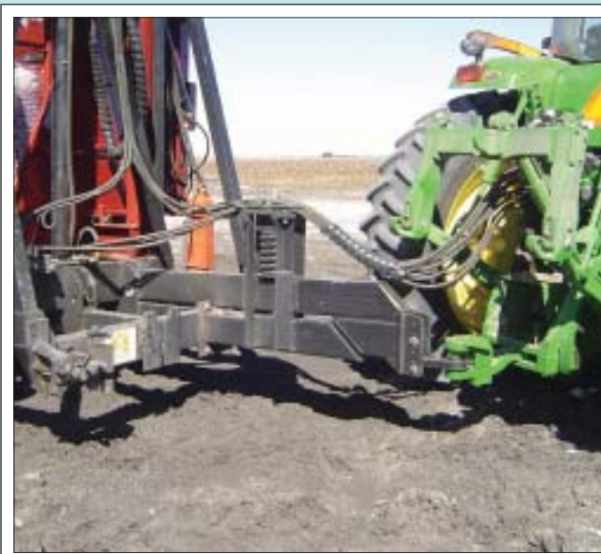
The cushion hitch makes for a smooth ride and reduced shock load.
