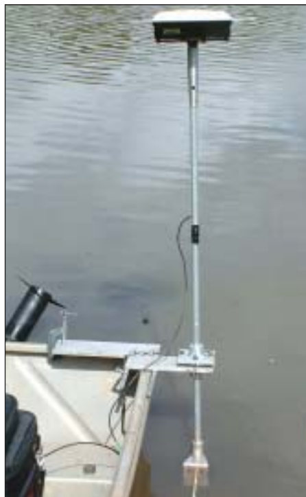
GPS antenna mounted above the electronic depth sounder.
