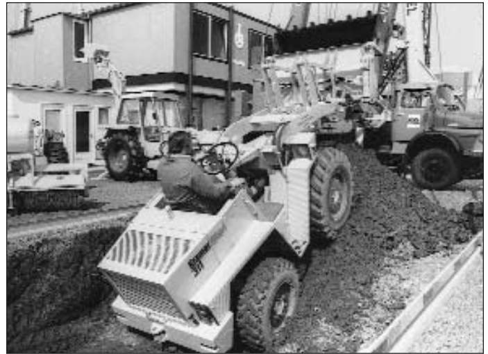
The Kramer 311 being put through its paces at the 1972 Hanover Trade Fair, was a well engineered four wheel drive unit. But the cost of adding a backhoe would have rendered it over priced for the Australian market. (Photo I.M.J.)
