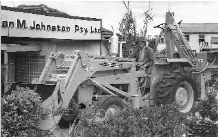
Manufactured in Britain, the Massey Ferguson loader/backhoe was Australia's top selling unit in 1972. The base tractor was a thinly disguised agricultural MF 35 with farm type brakes and transmission. Its performance on a work site was restricted by the two wheel drive configuration and driving in heavy traffic was dangerous, owing to the inadequate brakes and poor stability. Despite these short comings, which it shared with each of its competition, it was possibly the pick of the crop. (Photo I.M.J.)
