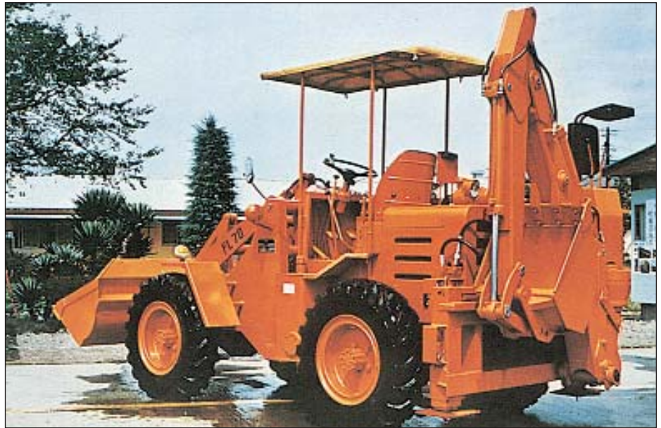
The Furukawa FL70 loader/backhoe was a brilliantly conceived industrial loader with a superb side shift backhoe that could be dismounted in two minutes. It featured four wheel drive, an articulated chassis, four speed fore-and-aft shuttle transmission, four wheel brakes and was powered by a powerful Isuzu diesel engine. (Photo courtesy Furukawa).
