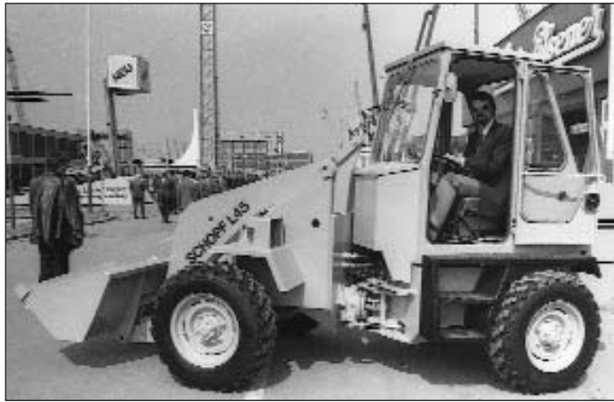
The well designed articulated Schopf T45 was eliminated as a contender, owing to its poor under-axle ground clearance.
