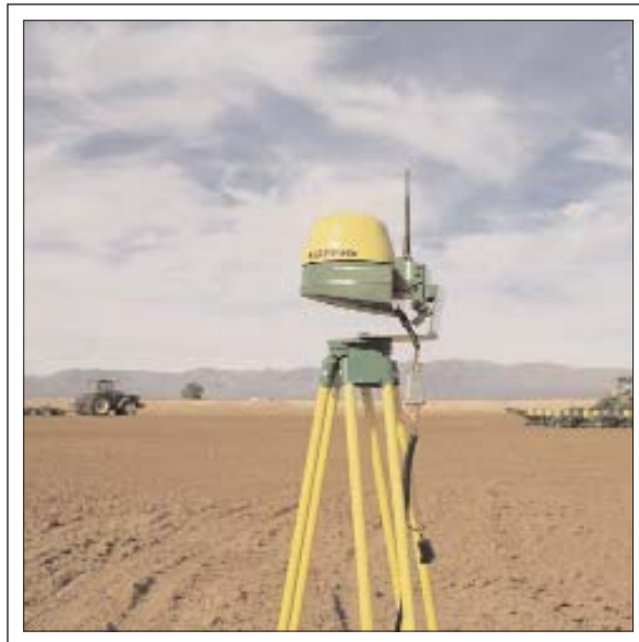
The Starfire RTK system has a ground-based reference station as well as a receiver on the vehicle.
