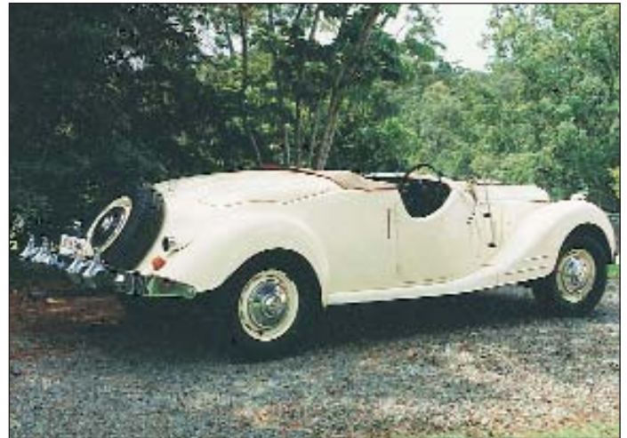
Taken from the rear quarter, this view of the Riley shows the hood down and the windscreen folded flat. During sports car race events it was common practice to lower the windscreen to obtain less wind resistance.
