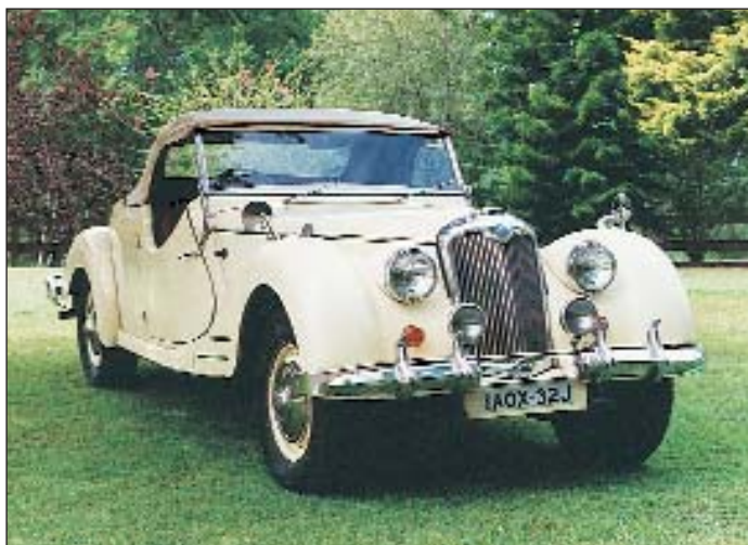
Photo is of the frontal view of the 1949 Riley Roadster showing the hood erected. The long bonnet conceals a high performance 2.5 litre twin cam engine. The same engine was used by Donald Healey in his race specials prior to his association with BMC and the Austin Healey.
