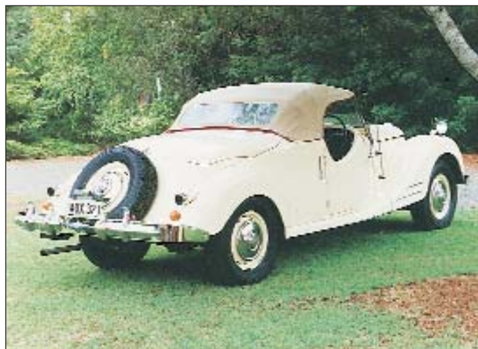
A rear view with the hood erected. There are also side curtains, stowed behind the rear seat, which can readily be put in place rendering the inside of the car completely dry in wet weather. The capacious rear boot is capable of accommodating several large suitcases plus a bag of golf clubs.
