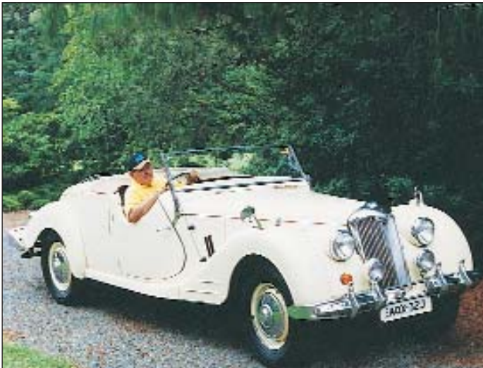
A frontal view with the hood folded, stowed and hidden beneath the tonneau cover. It takes no more than two minutes to either drop or erect the hood.
