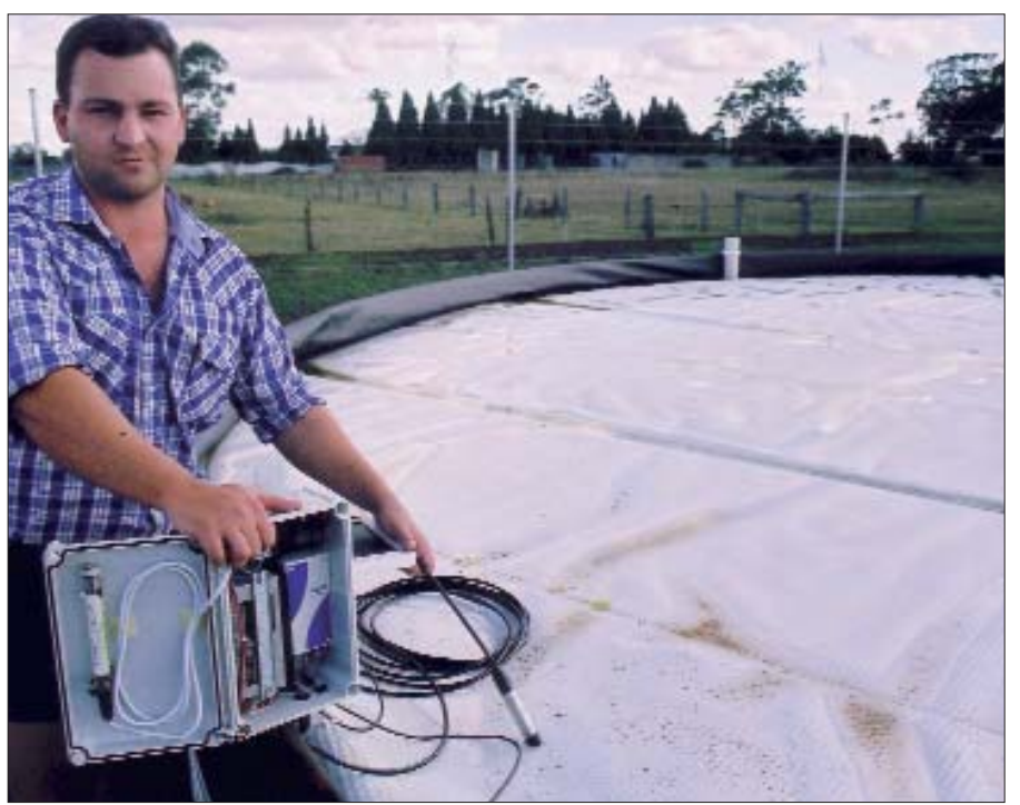
NCEA engineer Andrew Brier prepares this unique water pressure measuring kit to check evaporation control under EvapCap bubble wrap on 10 metre evaporation tanks.
