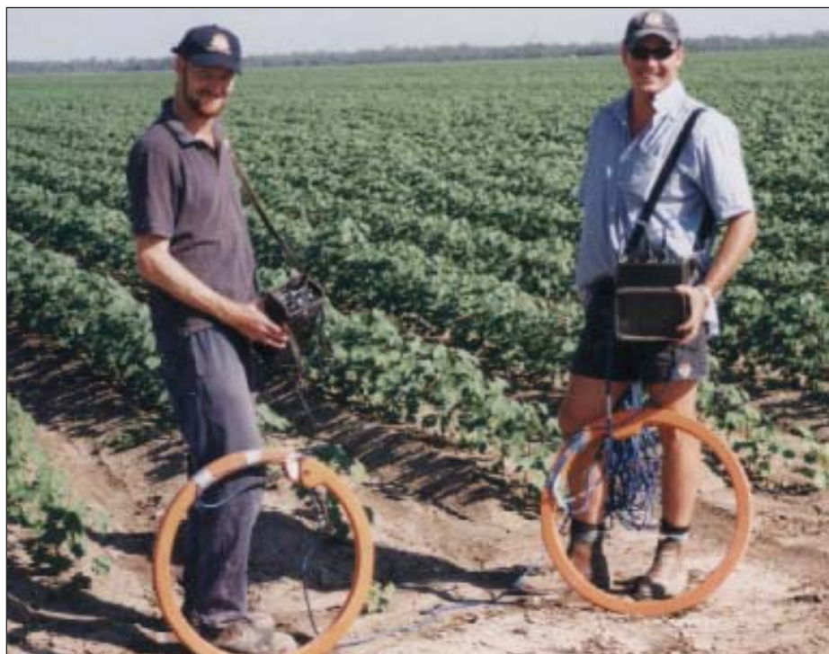
An EM34 instrument with transmitter coil and control (left) and receiver coil/control (right).
