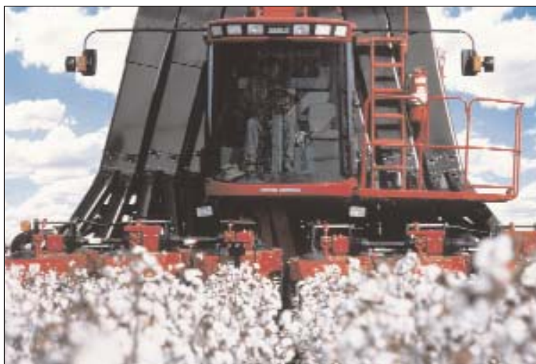
Like the first commercially successful mechanical cotton picker unveiled in 1943, the Case IH CPX610 cotton picker continues to harvest from both sides of the cotton plant for consistent harvest efficiency.
