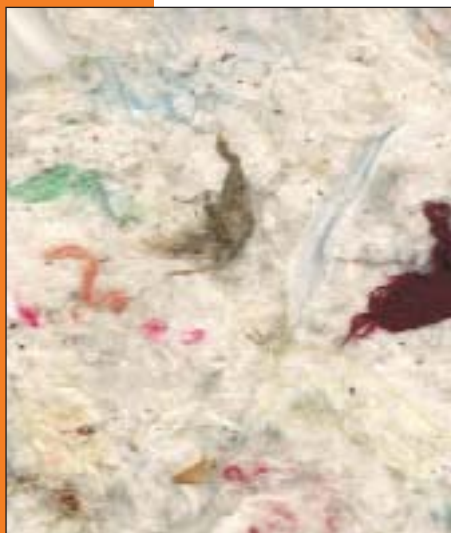
Examples of foreign material found in cotton bales delivered to spinning mills.
