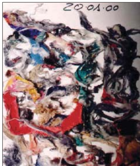
Examples of foreign material found in cotton bales delivered to spinning mills.
