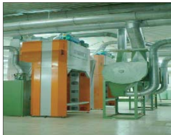
Blowroom equipped with Jossi detection systems.
