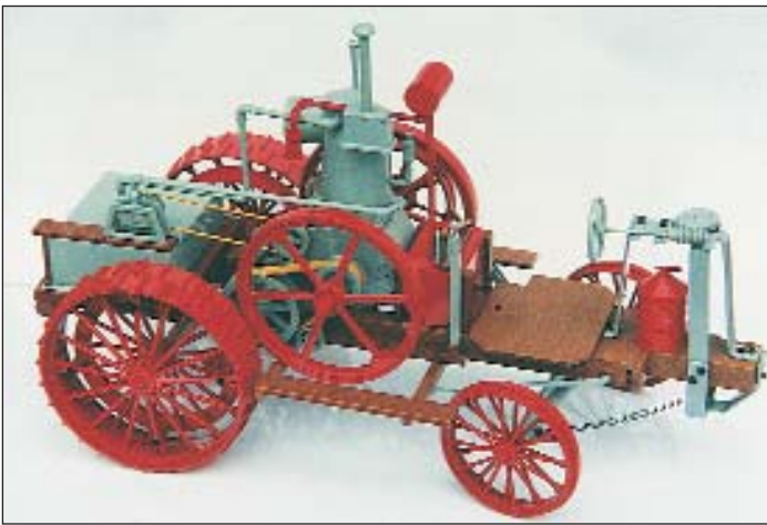
1892: The Froelich was powered by a Van Duzen vertical single cylinder engine with a bore and stroke of a whopping 14". It was considered that had the cylinder been placed horizontally, the end motion caused by the giant piston would have rendered the unit inoperable. Ignition was by a wet cell battery and contact points. (IMJ archives)
