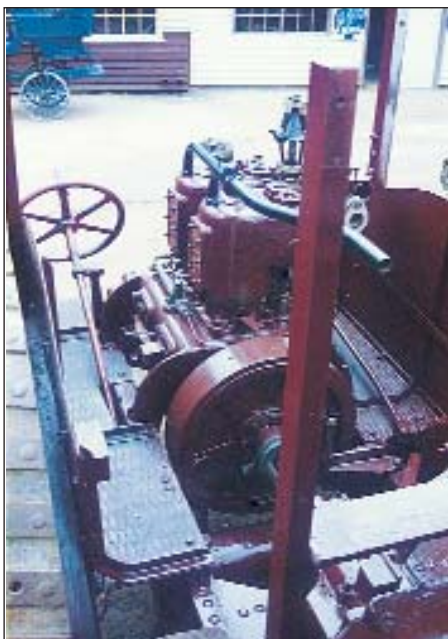
The engine of the Marshall Class C. Note the flying governor and the massive flywheel. The two cylinder unit produced around 30 hp. (Photo IMJ)
