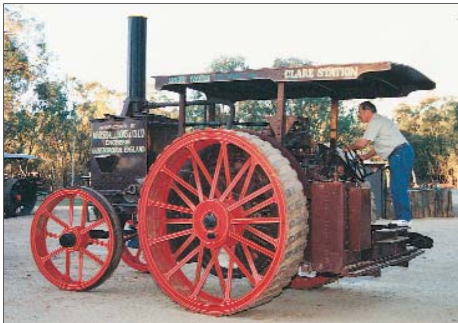
1909: Marshall and Sons of Gainsborough, England, introduced its Class C two cylinder tractor in 1909. The photo shows the author at the controls of a restored version owned by The Pioneer Village at Swan Hill, Victoria. The large tank above the front axle is a thermal siphon water cooling reservoir. The tractor was provided with a single speed gear. (Photo M. Daw)
