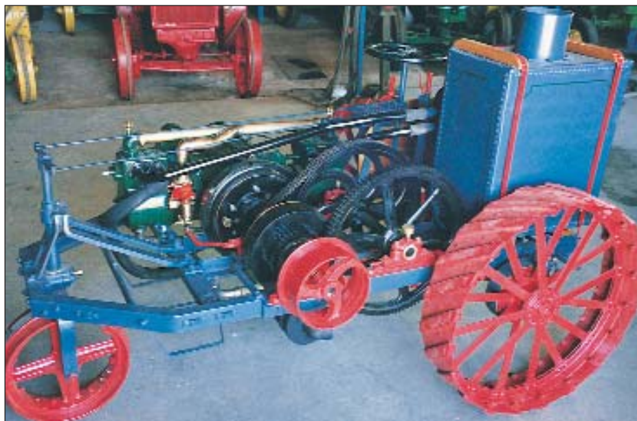
1903: The Ivel, produced by Dan Albone, bicycle manufacturer of Biggleswade, England, was a lightweight compared to the early American tractors. Powered by a two cylinder horizontally opposed water cooled engine, the Ivel was the first British tractor to be exported in volume numbers. The example pictured is Australia's oldest tractor and is owned by Norm McKenzie. (Photo IMJ)
