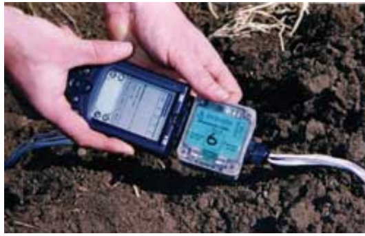
Initialisation and downloading of data from the advance meter is done with a Palmtop computer.
