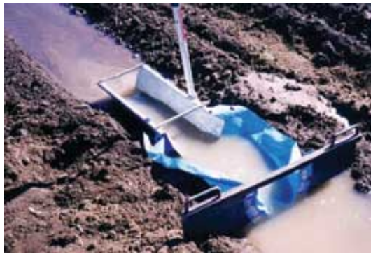
A flume located at the bottom of the field accurately measures tailwater.
