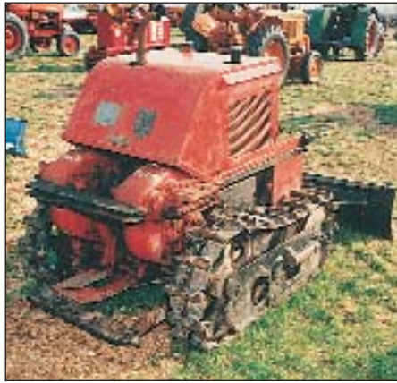
A 1949 Aveling Barford Calf Dozer owned by P and E Smith of Coalgate, New Zealand. The twin cast gearbox housings, each containing an over-centre clutch, are massively overbuilt for the nine hp engine. (Photo I.M.J.)
