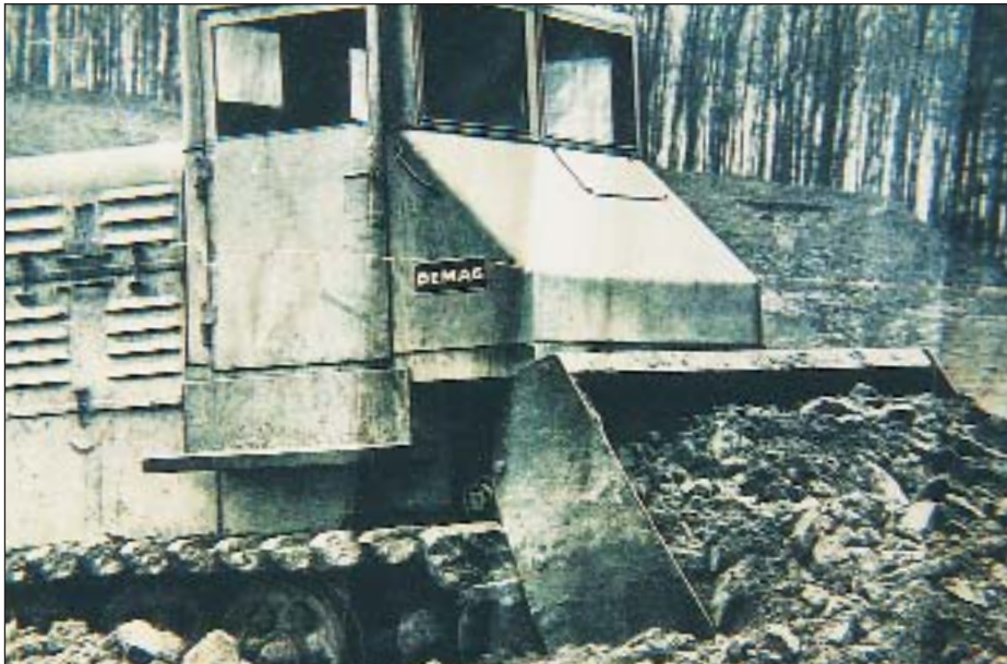
The Demag was surprisingly capable bulldozer, with no pretensions of looking beautiful. The big 12 ft dozer blade was operated by sensitive hydraulic controls, rendering it ideal for shaving or grading operations, demanding a high degree of accuracy. (Photo I.M.J. archives.)
