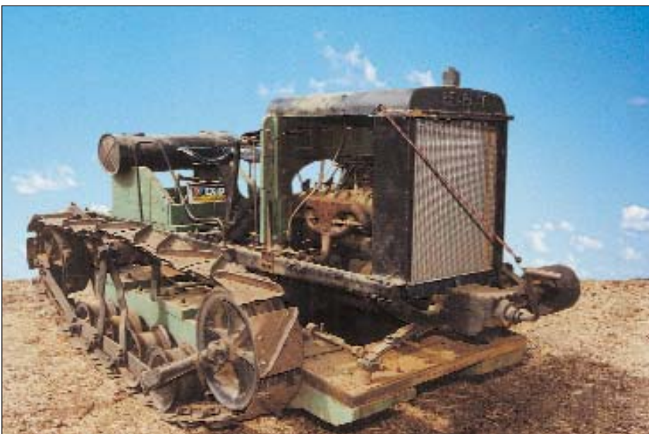
This 1923 Bearcat, owned by Lou Hanslow of Tasmania, spent its entire working life in Queensland. The wooden chassis is clearly evident. (Photo I.M.J.)
