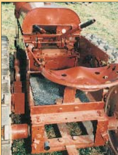
The only surviving Citroen Kegresse half track Polar tractor which took part in the unsuccessful bid to drive overland to the North Pole in 1934. The roller located in front of the vehicle was aimed at preventing the front wheels falling into an ice crevasse. (Photo I.M.J. courtesy Reynold's Alberta Museum, Wetaskawin, Canada.)
