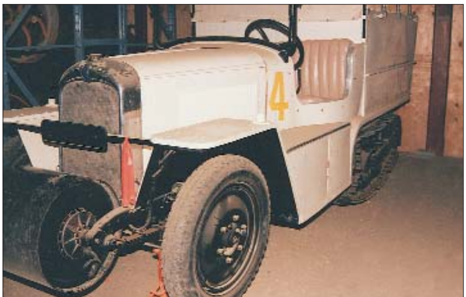
The only surviving Citroen Kegresse half track Polar tractor which took part in the unsuccessful bid to drive overland to the North Pole in 1934. The roller located in front of the vehicle was aimed at preventing the front wheels falling into an ice crevasse. (Photo I.M.J. courtesy Reynold's Alberta Museum, Wetaskawin, Canada.)
