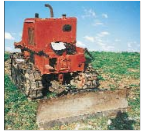
A front view of the Calf dozer showing the hazardous operator position. The levers at either side are the clutch controls and the front left lever is the control for raising and lowering the blade. (Photo I.M.J.)
