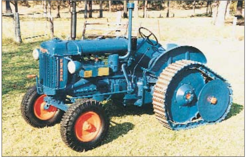
A 1949 Fordson/Roadless half track restored by the author. The four cylinder side valve petrol/kero engine of 4,380 cc delivered 32.5 belt hp and on half tracks produced a 6,000 lb drawbar pull at 1.54 mph. The unit was equipped with a three forward and one reverse gearbox. The operating controls were identical to that of the wheeled version. (Photo I.M.J.)
