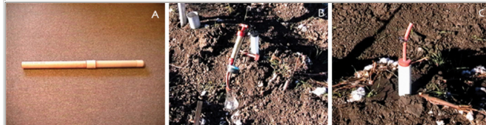
FIGURE 1: Ceramic cup samplers (A) used to extract soil water. The vacuum is maintained by a rubber stopper and tube sealed with a clamp (B). Soil water samples are removed by using a hand pump and a glass flask (C)
