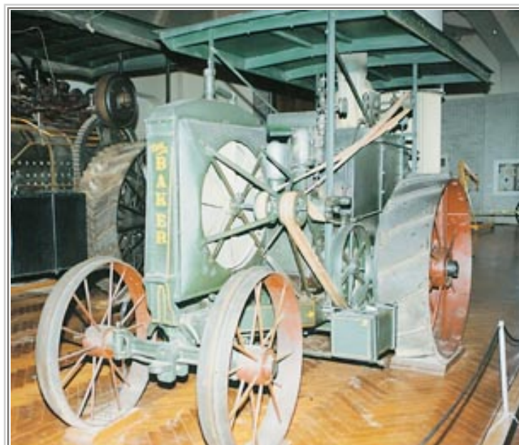
The Baker 16–30 steam tractor was introduced in 1921. It featured an automatic coal stoker and front mounted fan cooled condenser, which gave it the resemblance of a conventional tractor.
