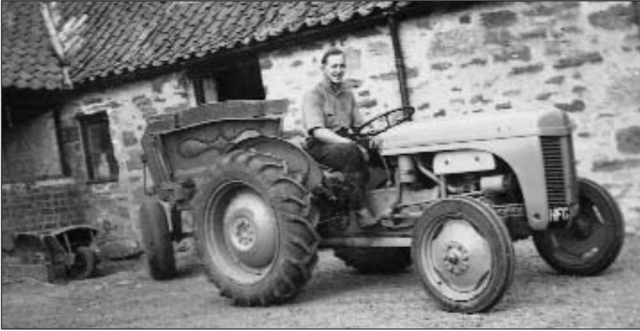
Pictured is the actual Grangehill Ferguson and trailer featured in the text. The Ferguson was a TED type which was fuelled on kerosene following a warm up period on petrol. The trailer was a converted horse cart equipped with World War II RAF bomber wheels and tyres. The driver is Willhugh Black. (Photo J. Black).
