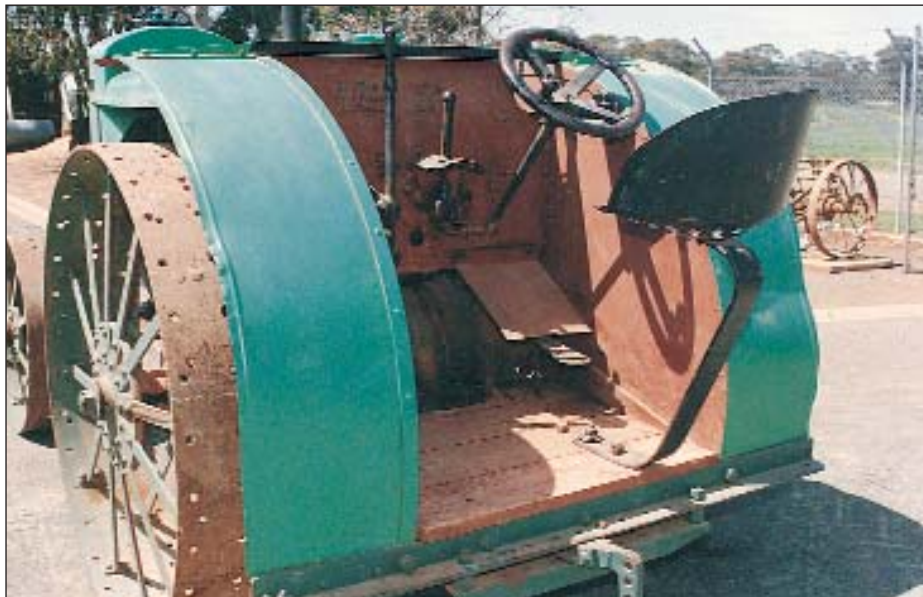
The rear view of a Super Drive at the Temora Rural Museum, NSW. The lever on the left is the hand clutch which, when eased forward, engages the drive but also acts on the governor control. The only other two controls are the gear selector and foot operated pulley brake. (Photo I.M.J.).
