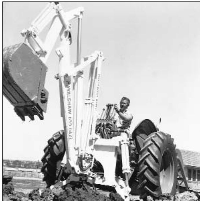
The Whitlock Dinkum Digger Mark 2 was manufactured in Australia in 1961–62. Note the depth and enclosed design of the standard bucket. In clay soil the operator would spend half his day with a crowbar endeavouring to clean out the packed clay from its innards. (I.M.J. archives).
