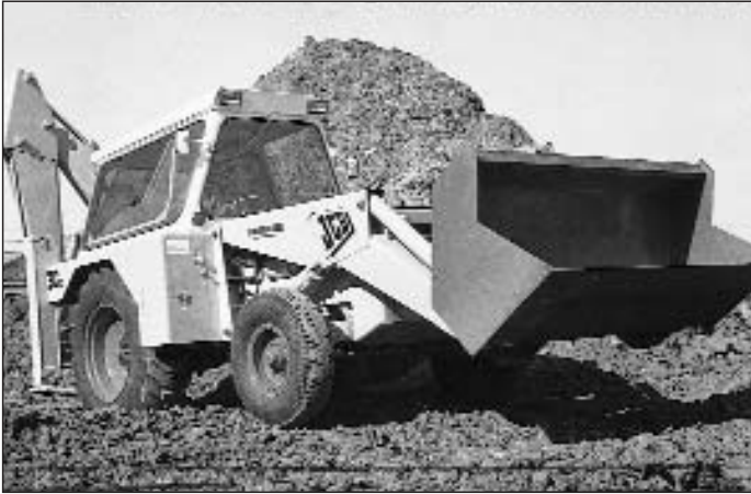
Lough Equipment Pty. Ltd. ditched the Whitlock in favour of JCB in 1956. As part of a global arrangement Blackwood Hodge Ltd. acquired the franchise in Australia a few years later. Pictured is a JCB 3Cii mounted upon a Leyland 4 cyl. diesel farm tractor. (I.M.J. archives).
