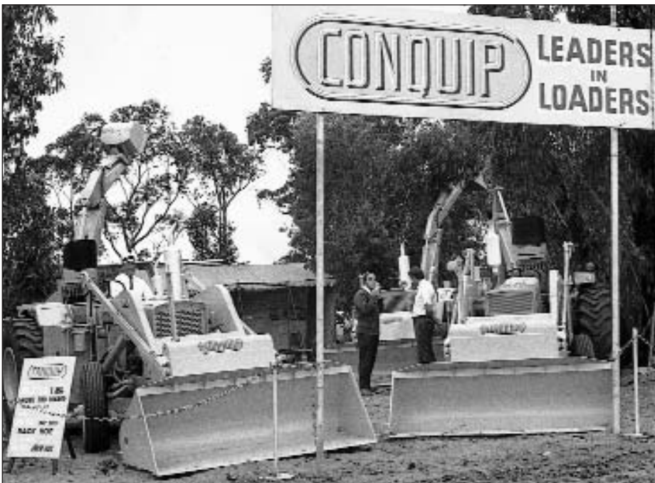
Conquip loader backhoes were the best of the Australian designs. The FEL 27 loader, with its parallelogram linkage, was the brain child of designer Sid Wild and a perfect match for the Chamberlain tractor unit. The BH 1 backhoe was powerful but slow and bulky. (I.M.J. archives).
