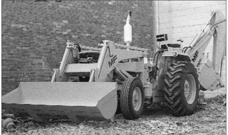
Massey Ferguson took the sales lead with its excellent loader backhoe, despite the fact that the tractor was basically a modified MF 135 farm tractor. Pictured is a 1969 MF 40. (I.M.J. archives).
