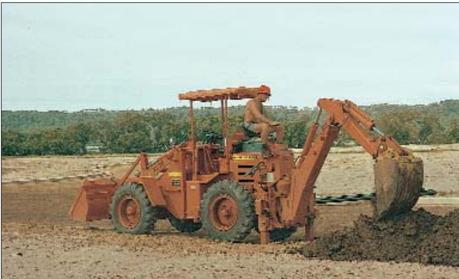
A Furukawa FL 70 loader backhoe shown working on the NSW central coast. This was the first tractor ever sold in Australia custom built from the ground up specifically as a base for a loader backhoe. It represented a breakaway from the outdated farm tractor philosophy. Warranty problems were negligible and the 4 cyl. Isuzu diesel provided an abundance of power. The 4 wheel drive and articulated chassis for this type of machine, was cutting edge technology. Imported into Australia by Ian M. Johnston Pty. Ltd. Rydalmere, NSW from 1971. (I.M.J. archives).
