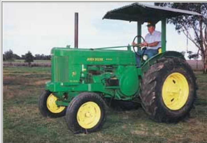
FOUR: Andrew Campbell, a grain farmer at Gulgong, NSW, has restored this 1956 John Deere 70. The two cylinder diesel engine is started by using a donkey engine of how many cylinders?
