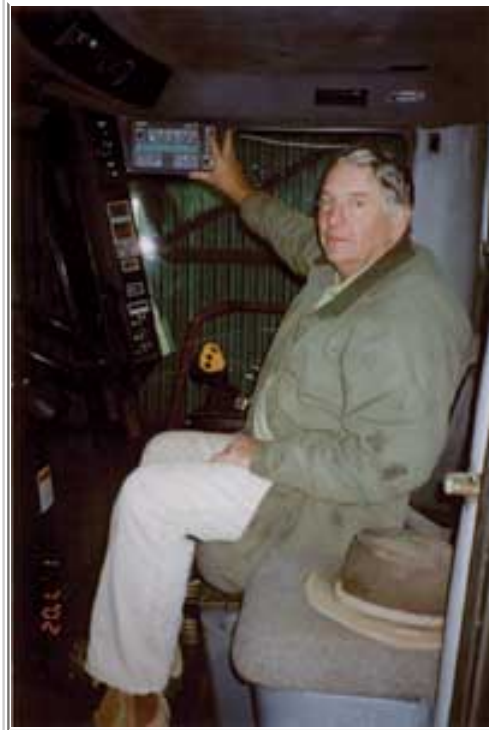
David Alexander adjusts the yield monitor in his grain header. The monitor links to a GPS sender on the roof of the cab and is fed data from sensors in the clean grain elevator.
