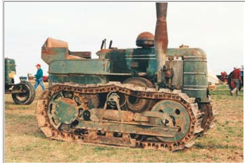
A 1949 Fowler VF Crawler owned by Stephen Arbuckle of Christchurch, NZ. Note the massive flywheel of the single cylinder compression diesel engine. The fitting at the lower front of the bonnet is for inserting a lit igniter for hand cranking. A wheeled Field Marshall, the stable mate of the Fowler VF can just be seen to the left of the photo. (Photo I.M.J.).
