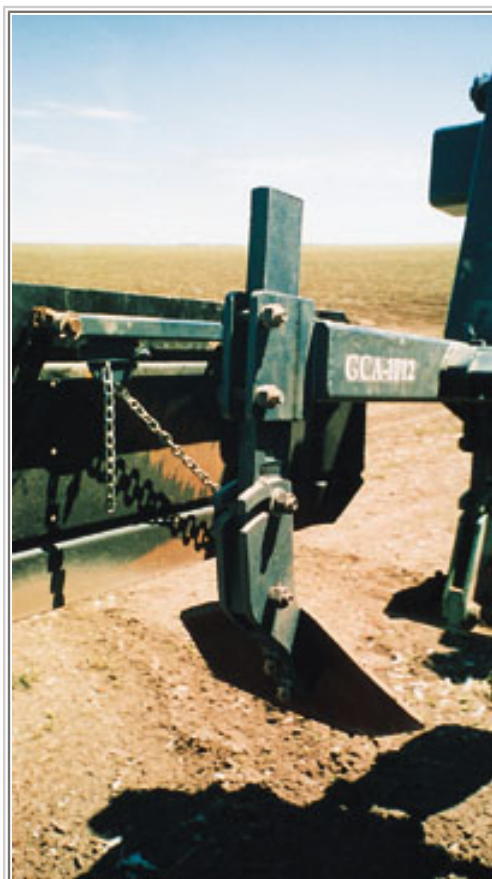
Simple rack and pinion shank depth adjustment on furrower
