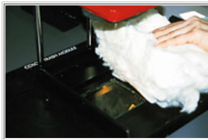
Sample placed for colour measurement with colorimeter and leaf grade with video trashmeter.
