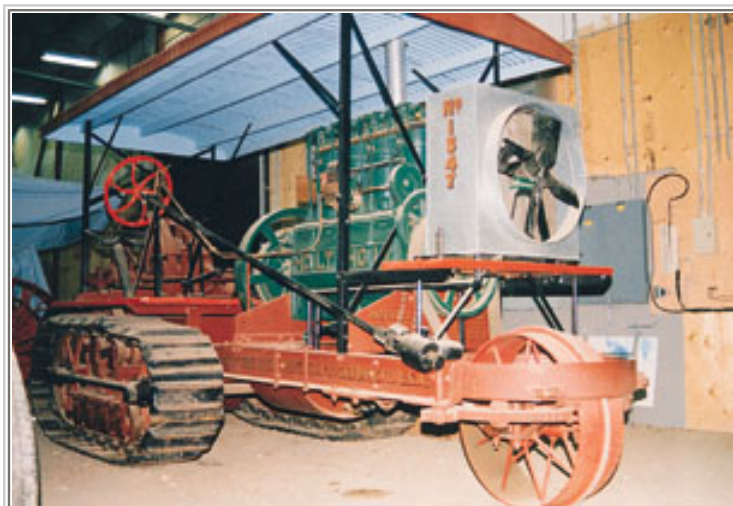
This 1910 60 hp Holt No. 1547 is a development of the firm's steam crawler patent of 1890. The four cylinder petrol engine had an exposed clutch and flywheel and was lubricated by a Maddison Kipp metering type oiler. It also featured high tension ignition and fly ball governor. (Photo I.M.J. taken at Reynold's Alberta Museum, Wetaskiwin, Canada).
