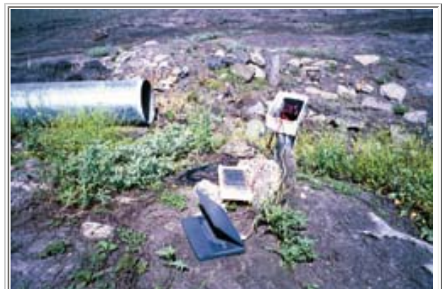
The Starflow logger and laptop take data from the instrument.
